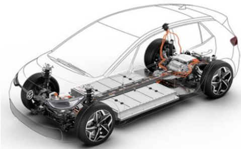
The location of lithium-ion battery pack in an electric vehicle (i.e. Volkswagen ID.3)
