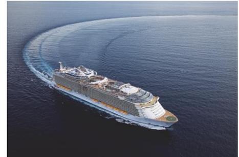
“The **advance** should **not exceed 4.5 ship lengths (L)** and the **tactical diameter** should **not exceed 5 ship lengths** in the **turning circle maneuver**.”
